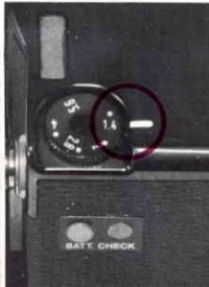
**11** When the lens speed adjustment dial is turned, the f/stop scale of the meter reading window slides and the lens speed is indicated just below the under-exposure warning mark as a maximum f/stop.
